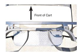
3. Align a straight edge with the center of the welded in nut on the Golf Bag Attachment Bar and mark the outside of the armrest. This will be the center of where you drill.
