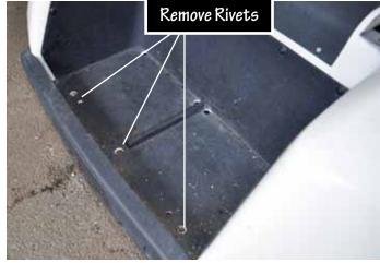
5. Using a 1/2" drill bit, remove bag well rivets. 4
