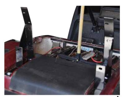
6. Set in rear seat supports and line up holes in supports with those where basket bolts were removed in step 4. Use hardware in pack #4 to attach seat supports to vehicle.
