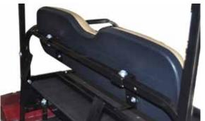
13. Attach seat back cushion to horizontal bar bracket using hardware from pack #2.
