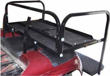
10. Attach Horizontal Support Bracket and Armrests using hardware from packs #3 and #7. You will need the remaining hardware in pack #3 in the next step. Do not tighten hardware.
