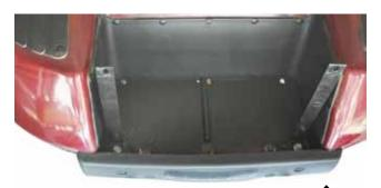
7. Attach seat frame support brackets using hardware from pack #2.
