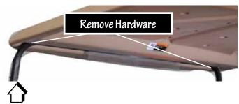
1. Remove all canopy hardware (nuts, bolts and washers) from 4 corners (2 in front and 2 in rear) of vehicle canopy. Retain the hardware. You will need them to reattach canopy to vehicle.
