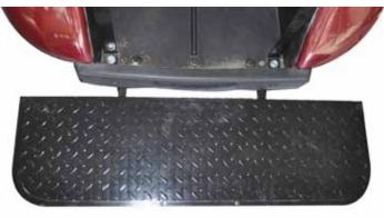
8. Attach footrest with hardware in pack #5 in 3places where bag well rivets were removed.
